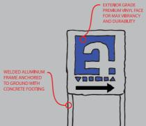
SIGN FACES ATTACHED DIRECTLY TO ALUMINUM FRAME FOR CLEAN LOOK AND MAX DURABILITY
